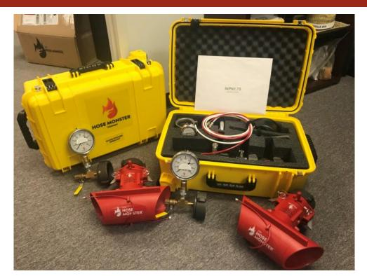
There are few limitations to what equipment can be used to test fire pumps. The general requirement is that the pressures and volumes are achieved. It is important to ensure that you are using quality equipment such as calibrated gauges and that the flow testing equipment is not faulty. This can lead to inaccurate information and failing fire pump results. Section 8.3.3.5 outlines testing equipment and below is a link to a blog regarding calibration of gauges and other testing equipment.
